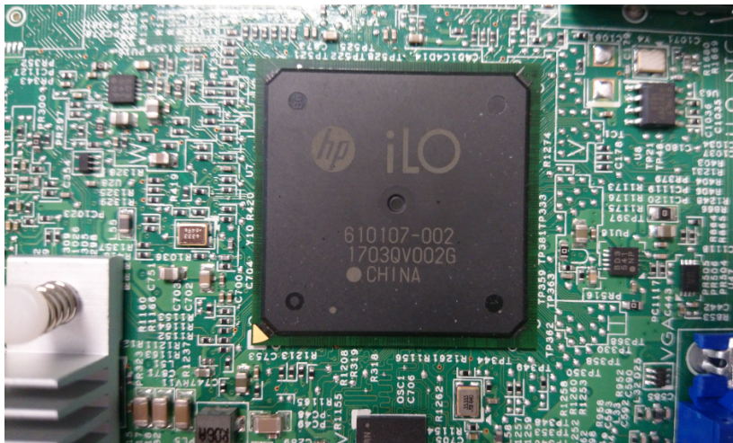
Figure 1: Directly integrated in the server's motherboard
